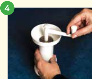
Insert handle/cutter and rotate handle while pressing slowly downward.
